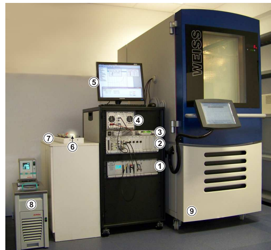
Photo of the Viking Reliability Tester (VRT) with the measurement setup used for pre-stress LED evaluation
